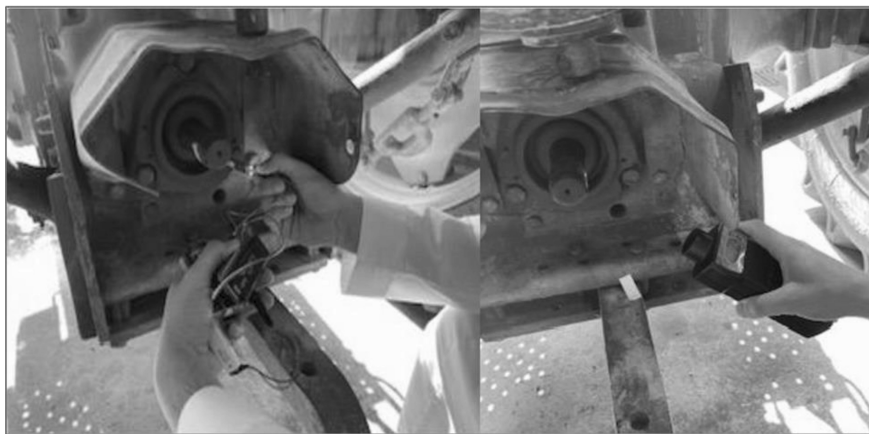
Fig. 5. Measuring the rotational speed by the designed module and a commercial Tachometer rpm counter on the tractor rear power take-off shaft (PTO).
