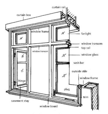
Fig. 8. Engineering structure of the casement window.
