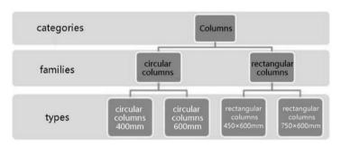
Fig. 9. The system structure of the Revit software.
