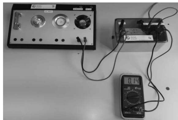
Fig. 3. Setup for current measurement on the fan.
