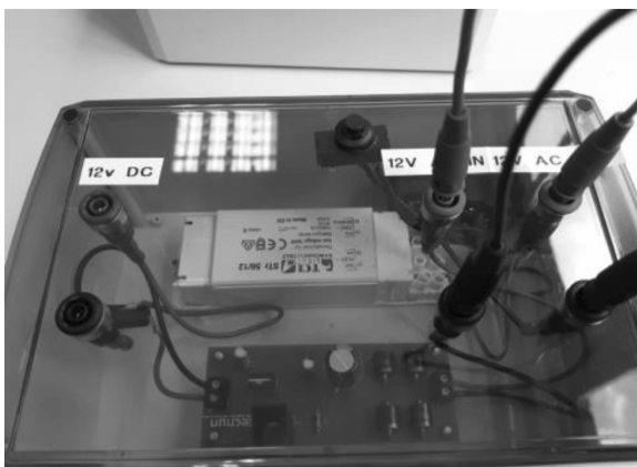
Fig. 2. 230 to 12 V AC/AC and AC/DC converters with magnetothermic switch.
